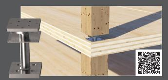
PILLAR allows the construction of floors with column-to-floor system without beams, without the need of special connections between panels and with free spans greater than  $3.5 \times 7$  m.
